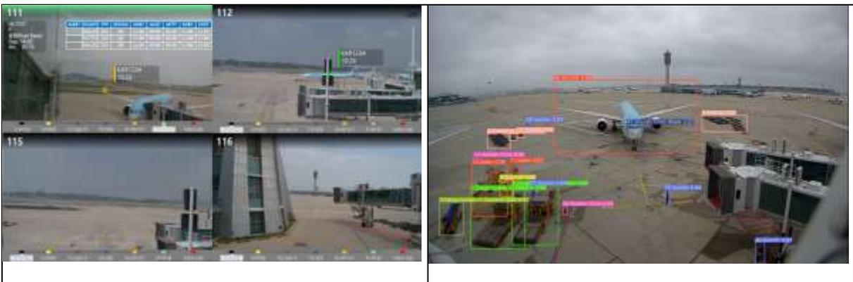
2.4 The entire apron area of Incheon Airport is digitally transformed into a 3D model, creating a digital twin. Within this digital twin, real-time information, such as aircraft identification, location, and gate status, is displayed to support air traffic control operations.
