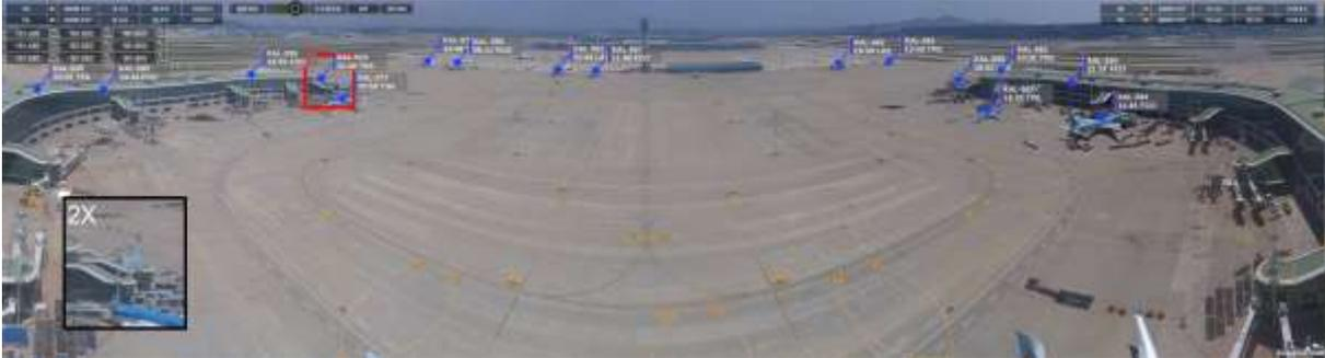
2.3 To monitor the operational status of the aircraft at a gate, the system automatically switches and displays either the departure or arrival gate, as needed.
