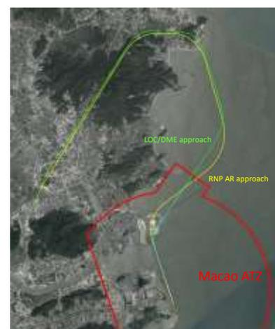
Figure 1 - Flight tracks of LOC/DME and RNP AR approach procedures
